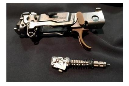
Although SIG was already working toward introducing the MHS-inspired Enhanced Trigger to the P320, this -30deg drop issue has hastened their effort. They have lightened the Trigger, Striker and Sear by about 30% overall and added a Disconnect (commercial only, not MHS). The trigger pull weight is unaffected, but rather the trigger part actually weighs less. The reason they lightened those parts is to mitigate the momentum gained by the heavier parts during a drop.
